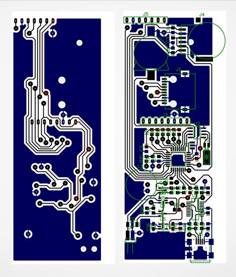
Fig 1 Contactless Attendance Logger – PCB design
