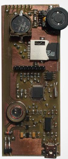
Fig 1 Contactless Attendance Logger – final product and bare PCB with components
