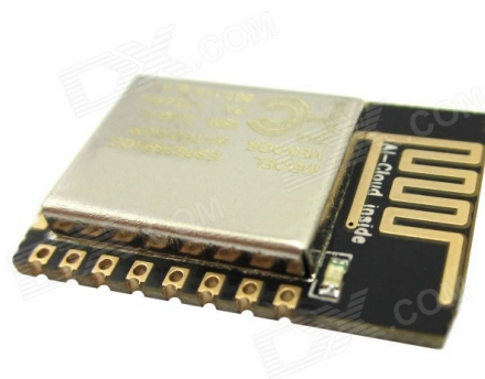
Figure 4–2 The certified ESP-12E module exposing all GPIOs
