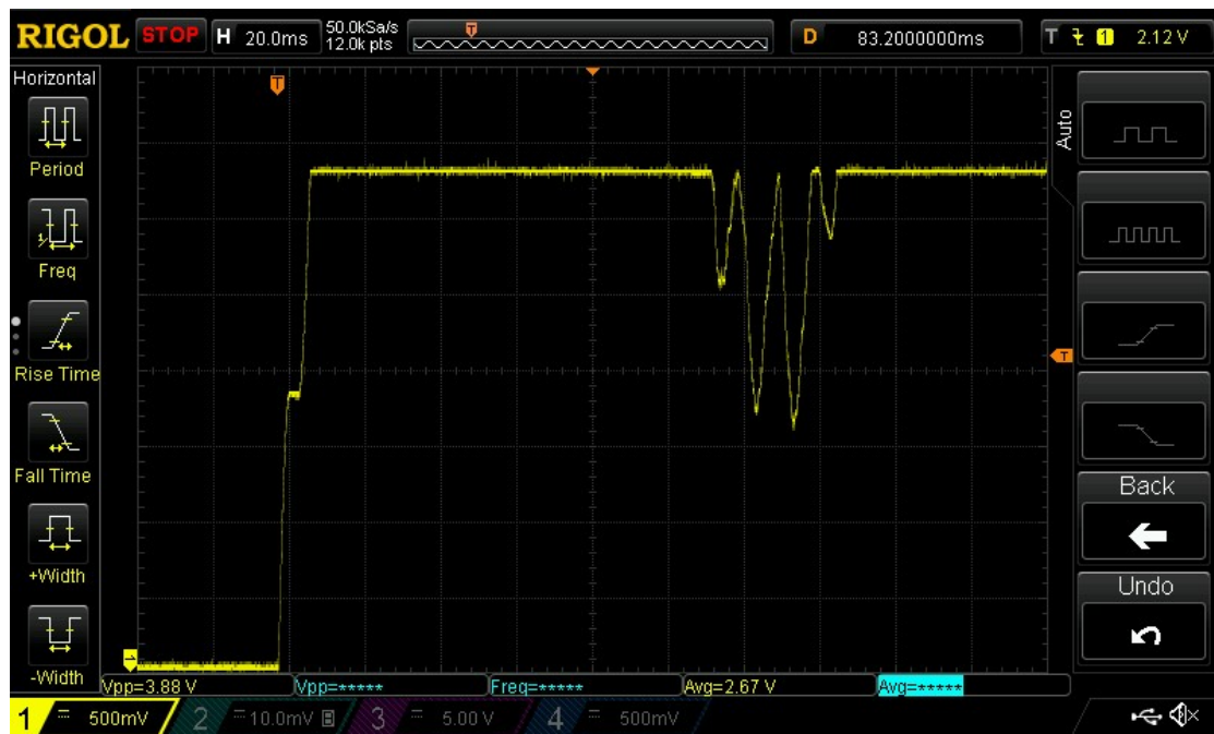
Figure 7–2 The power line of the ESP-12E inspected during the boot-up by the oscilloscope - it looks the same either if the processors boots, or it doesn't, suggesting the possible occurrence of the ESP8266 firmware problem
