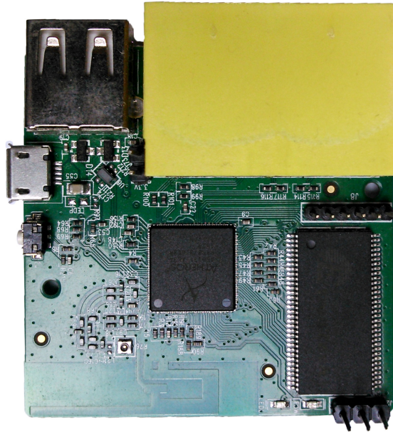
Figure 3 – 2 The front side of the GL.inet board exposing the main Atheros SoC, RAM and interfaces
