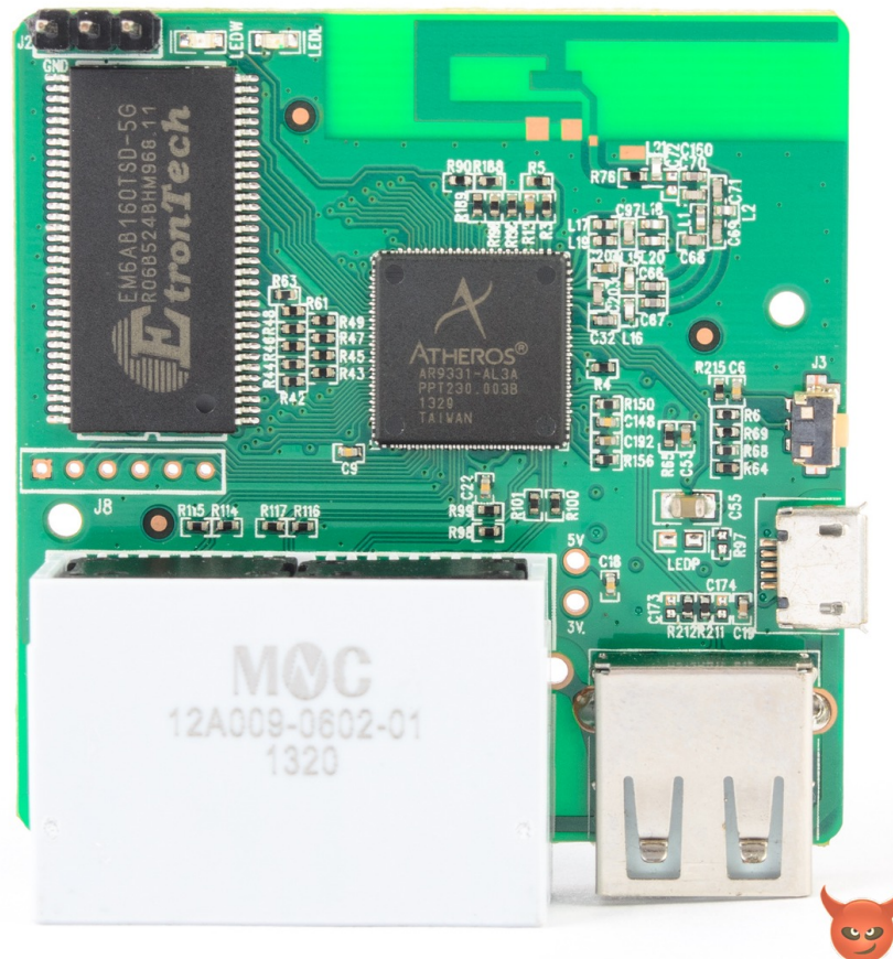
Figure 2–2 The front side of the GL.inet board exposing the main Atheros SoC, RAM and interfaces
