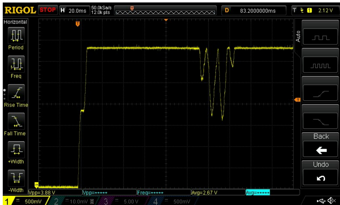
Figure 7–3 The power line of the ESP-12E inspected during the boot-up by the oscilloscope - it looks the same either if the processors boots, or it doesn't, suggesting the possible occurrence of the ESP8266 firmware problem
