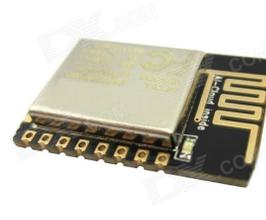
Fig. 4. The certified ESP-12E module exposing all GPIOs
