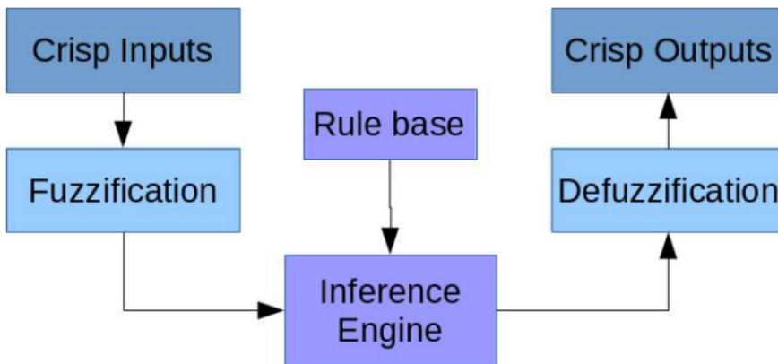
Figure 10: Block diagram of a fuzzy control
