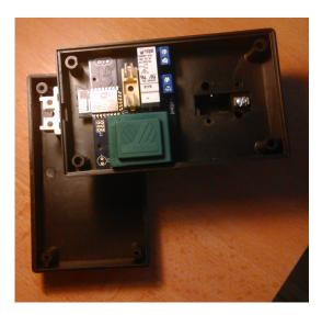
Fig. 10. The view into the client node's enclosure, before the final assembly, exposing top side of the board containing linear transformer T1 (green), mains connectors J1 and J2 (blue), a fuse holder for F1 (yellow-ish), a relay K1 (white) and an ESP-12E module
