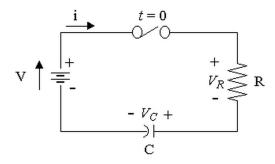
Fig. 7. RC circuit diagram.
