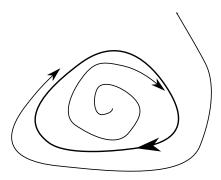
Fig. 1. Stable limit cycle. Trajectories spiral towards it.
