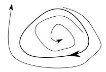
Fig. 2. Unstable limit cycle. Trajectories spiral away from it.
