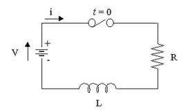
Fig. 6. RL circuit diagram.
