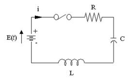
Fig. 8. RLC circuit diagram.
