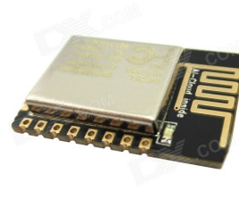
Fig. 4. The certified ESP-12E module exposing all GPIOs
