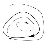
Fig. 3. Half-stable (or semi-stable) limit cycle. Attract trajectories from one side and repel them from other side.
