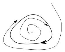
Fig. 1. Stable limit cycle. Trajectories spiral towards it.
